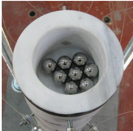
Figure 4: Particle damper (diameter of hollow part = 80 mm)
