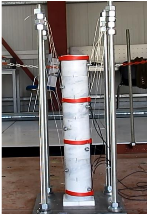
Figure 1: Column-model with safety structure.
