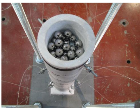
Figure 5: Damper with large diameter hollow part containing steel spherical particles.
